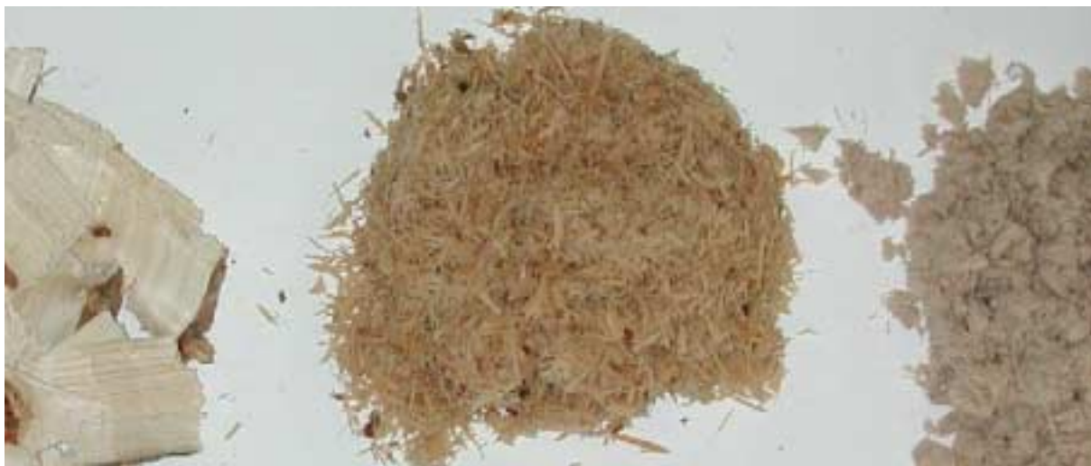
Figure 6: Tornado fibre (centre) has a high percentage of high length-to-diameter ratio fibre bundles with a minimum amount of fines. Conventional chips (left) and refined pulp fibres (right) are for reference.
