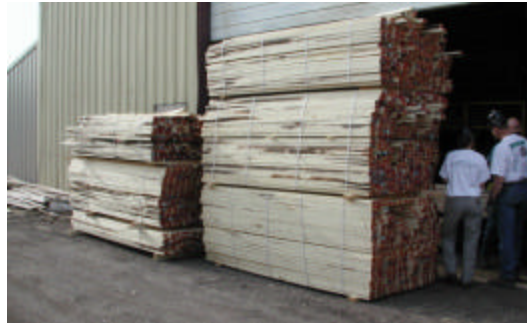
Figure 5. Over 1000 2x4 material E-rated according to low, medium, and high dynamic Modulus of Elasticity and ready for fabrication into laminated I-beams.
