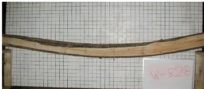
Figure 3. Example of a 6% curve d small tree cut horns-up through a conventional band saw.
