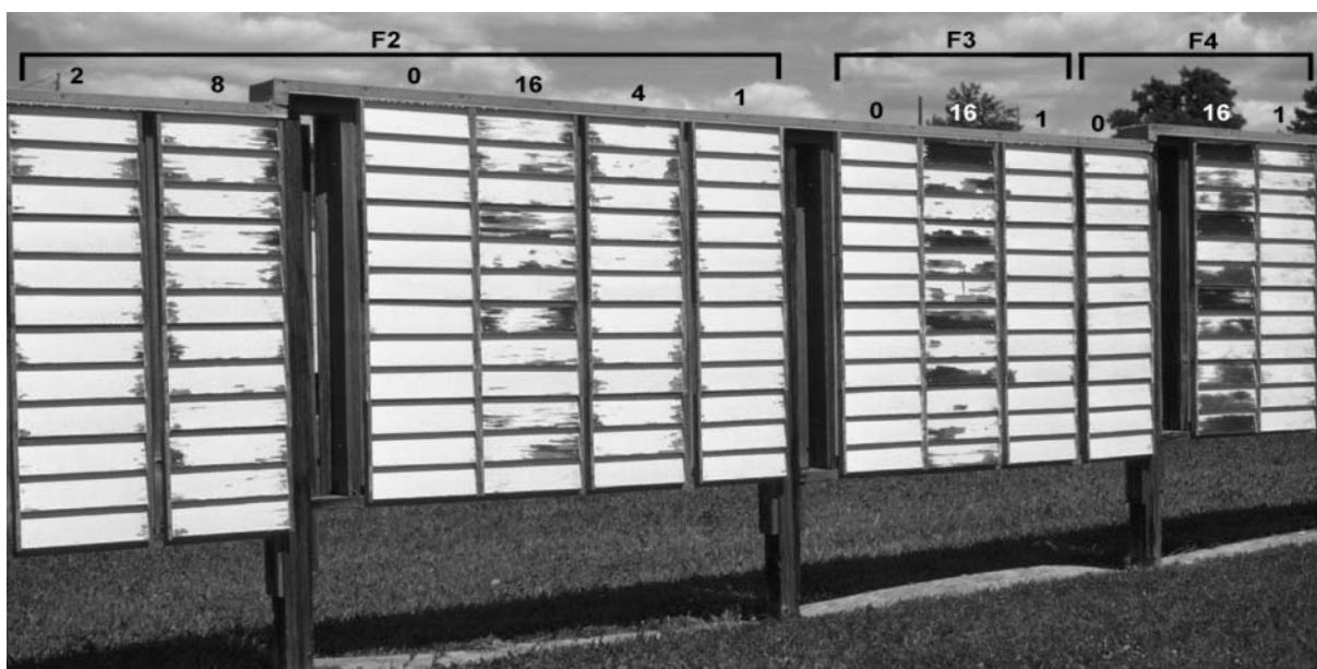
Figure 7. Exposure fence west of Madison, Wis., showing painted specimens after 17 years of outdoor exposure (F2, WRP/alkyd/latex; F3, alkyd/latex; F4, latex/latex; numbers are weeks of preweathering).
