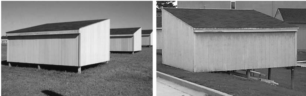
Figure 7. Field chambers for monitoring roof temperatures in Wisconsin on left (northern U.S., 43.4°N) and Mississippi on right (southern U.S., 33.5°N).
