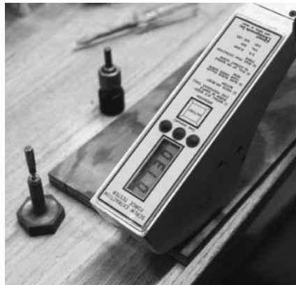
Figure 5. Screw-pull test using hand-held load cell.
