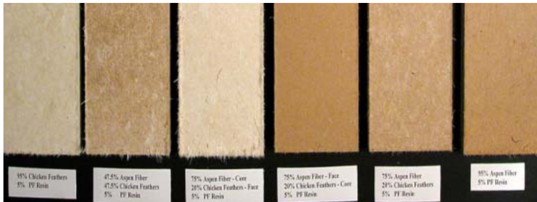
Fig. 1 various combinations evaluated of aspen wood fibre and CFF,
