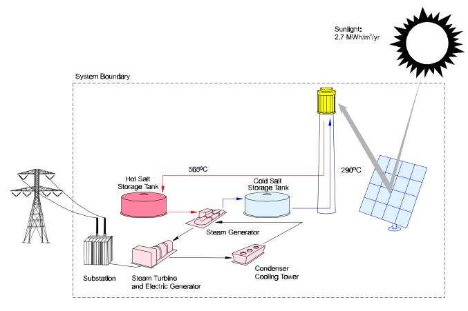
Figure 1. Molten-salt power tower system schematic (Solar Two, baseline configuration).
