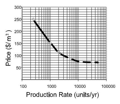
Figure 7. Heliostat price as a function of annual production volume. These prices apply to a heliostat with a surface area of 150 m<sup>2</sup> and similar in design to those tested at Sandia National Laboratories.
