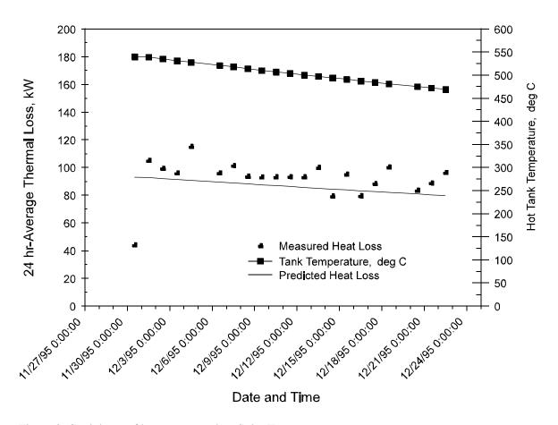
Figure 3. Cool down of hot storage tank at Solar Two.
