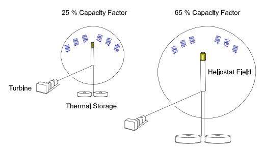
Figure 6. In a solar power tower, plant design can be altered to achieve different capacity factors. To increase capacity factor for a given turbine size, the designer would (1) increase the number of heliostats, (2) enlarge the thermal storage tanks, (3) raise the tower, and (4) increase the receiver dimensions.
