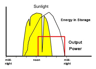
Figure 2. Dispatchability of molten-salt power towers.
