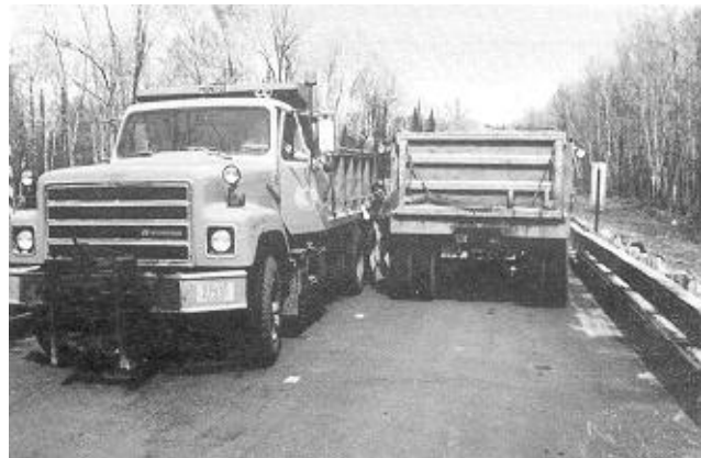
Figure 19—Load position 3 with both vehicles on the bridge. (M92 0009-13)
