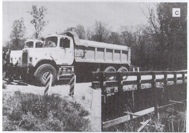
Figure 15—Vehicle load test positions: (a) load case 1, span 2; (b) load case 2, span 2; (c) load case 3, span 1.
