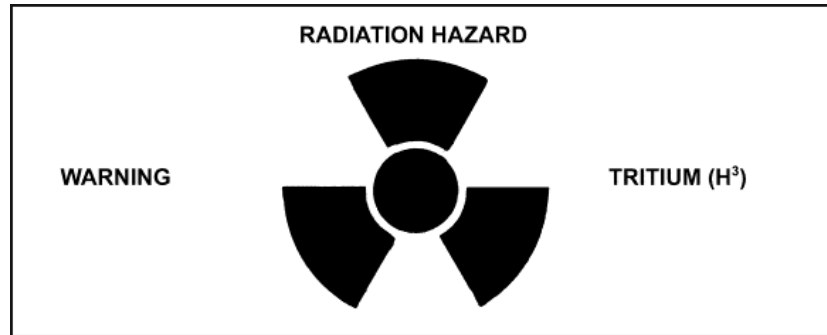
Figure 2-14. Warning label for tritium gas (H 3 ).
