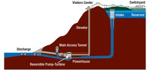
During periods of low power demand, the pump-turbine pumps water up into the mountaintop reservoir. During periods of high demand, water from the reservoir flows down through a tunnel drilled into the mountain, driving the generators in the underground power plant.
