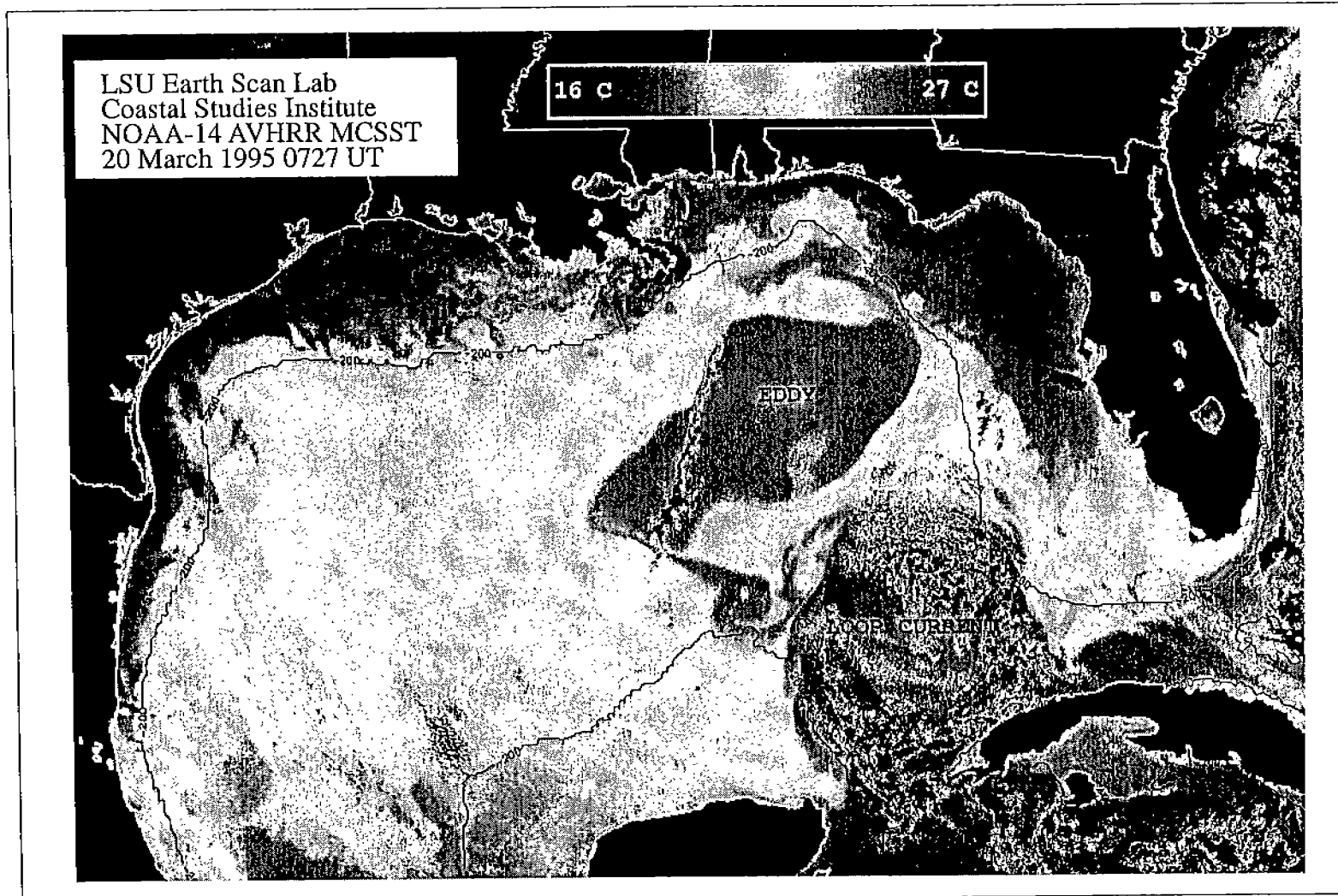
Figure 4. AVHRR image (20 March 1995) showing Loop Current extending into the southeastern Gulf with newly detached Eddy Z (courtesy of Nan Walker, Louisiana State University).
