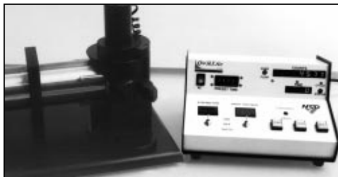
Figure 1. QwikLite bioassay system. On the left, the PMT is bolted to the test chamber. The controller box, on the right, provides power to the PMT, stir motor, and displays PMT counts.
