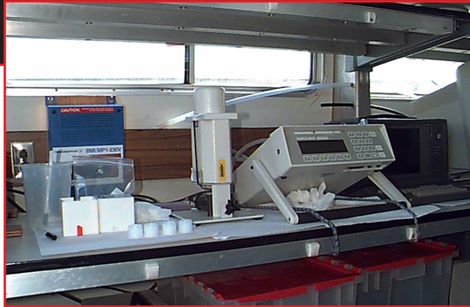
Field portable x-ray fluorescence for on-site measurements of metals in sediments on board survey craft
