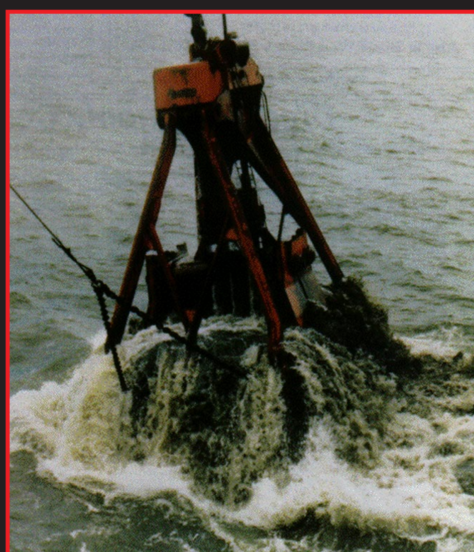
Clamshell dredge may cause contaminant suspension and release—sediment characterization can predict potential impact
