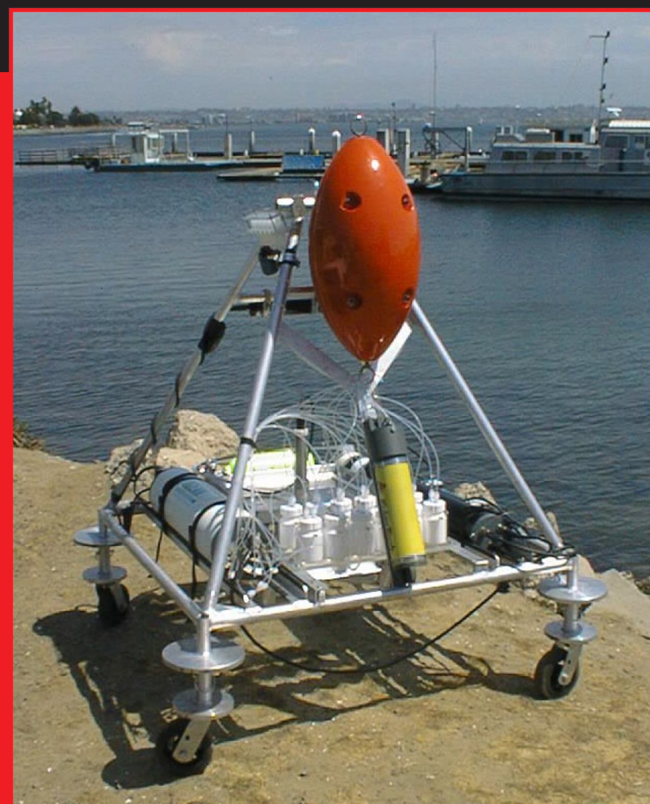
Commercialized Benthic Flux Sampling Device for in-situ measurement of contaminant transport into or out of sediments
