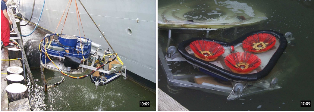
Figure 14. View of the AHMV at work (left) and underside of hull-cleaning brushes (right).
