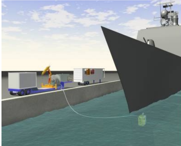
Figure 16. Artist's rendition of the underwater hull-cleaning system and mobile support modules.
