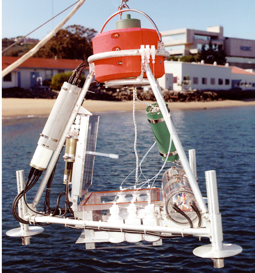
Figure 35. Benthic Flux Sampling Device (BFSD).
