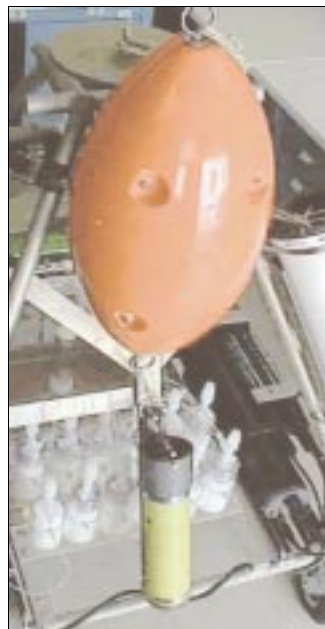
Figure 13. Acoustic release and retrieval buoy.
