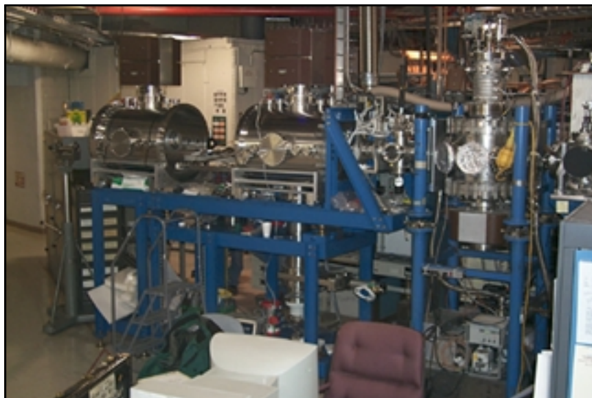
Instrumentation and chamber on the NRL X24C beamline at the National Synchrotron Light Source, Brookhaven National Laboratory
