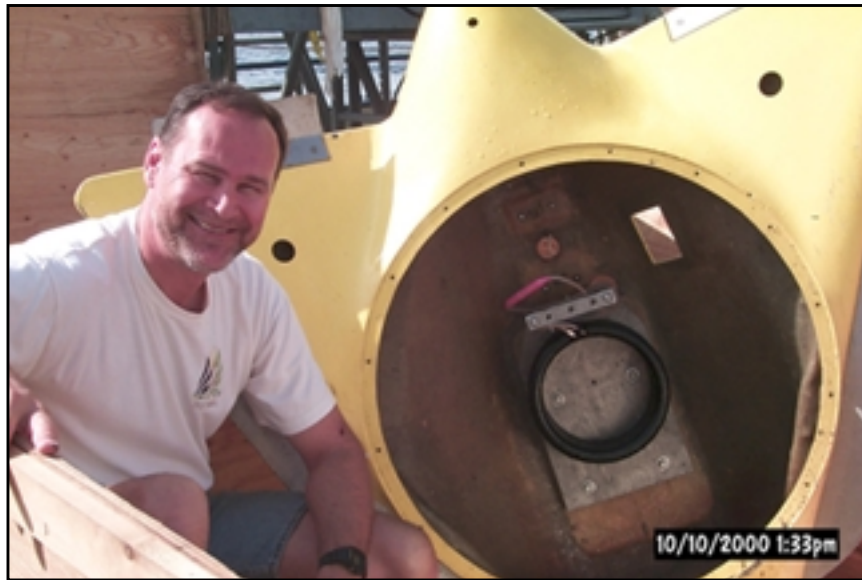
200 dB source transducer and V-fin towbody
