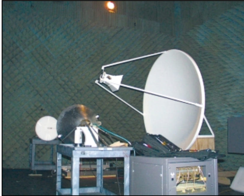
12-ft antenna dish in the Isolation Measurement Chamber
