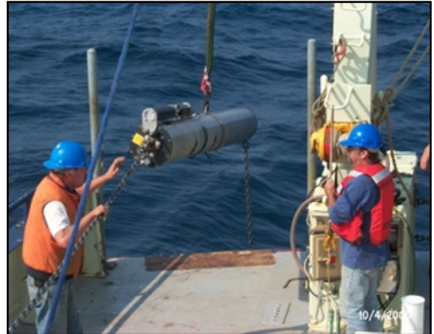
RF-telemetered receiving array (left) and an autonomous sound source (right) being deployed in the ocean
