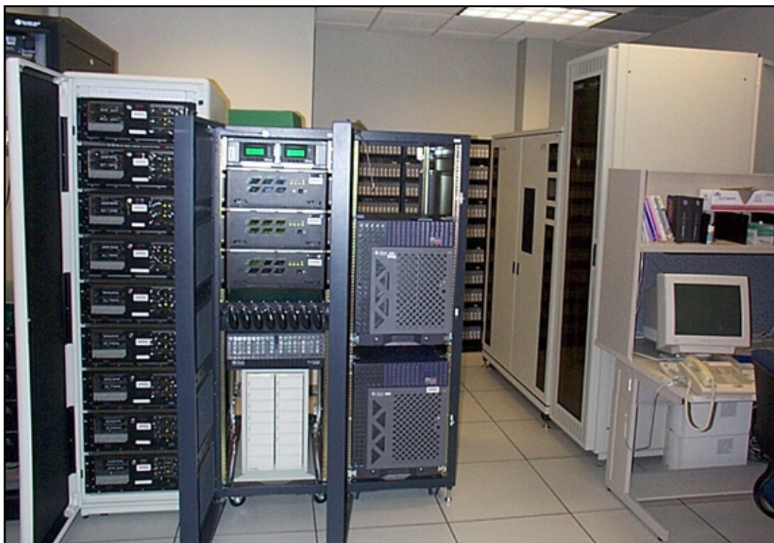
Central elements of the Sun and Alpha Workstation clusters, and DLT tape library
