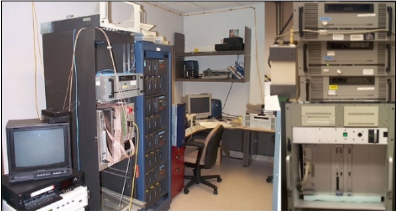
Radar Imaging Facility Raid Storage System, real-time processor, and VLDS recorder units
