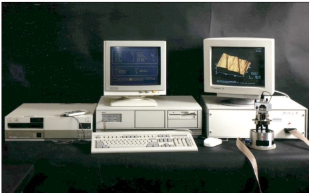
Main components of the atomic force microscope
