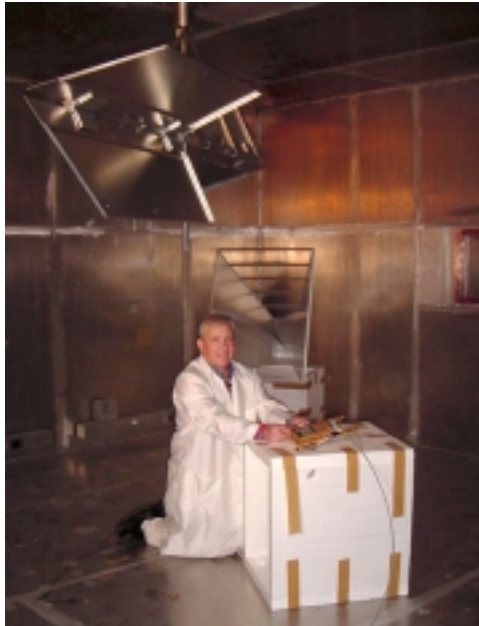
Transmit/receive module assembly undergoing a radiated susceptibility assessment
