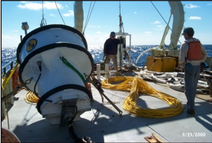
RF-telemetered receiving array (left) and an autonomous sound source (right) being deployed in the ocean
