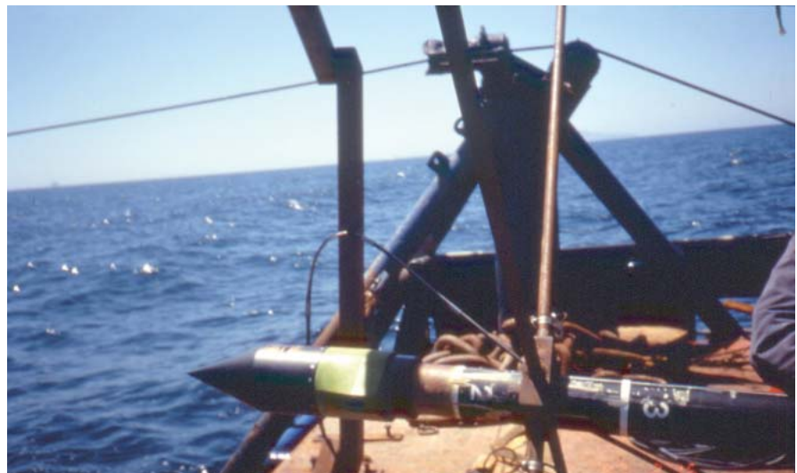
Above: The SEMS project consists of three seismic probes embedded into the seafloor and wired to computers on nearby platforms. Below: A probe can record a magnitude 4.0 earthquake within a 25-mile radius.
