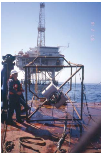
Left: Installation of seismic probe near Platform Grace.
