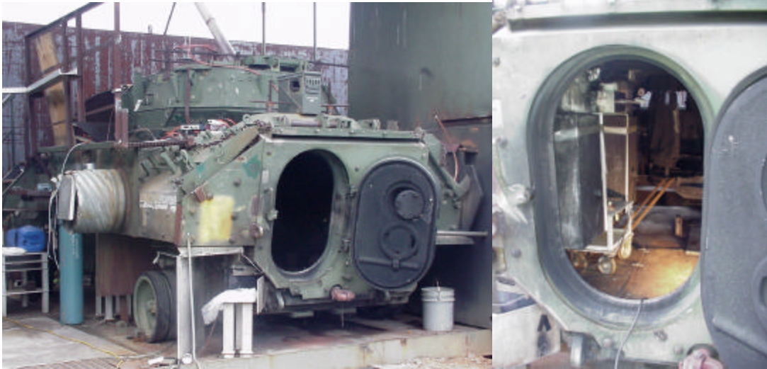
Figure 20. (a) Modified Bradley Armored Personnel Carrier; (b) Head Height Location of the DIRRACS-II, Set Between Two “Occupants”
