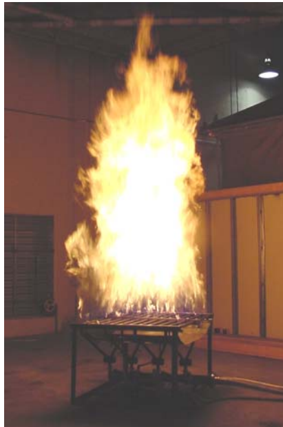
Figure 9 Photo of 3 MW fire from the natural gas burner.
