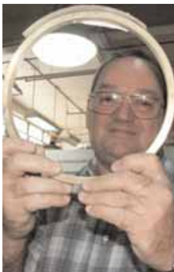
ABOVE: Quality Inspector Milton Amos inspects a main oil-pump ring for Shawnee Fossil Plant before it is shipped to the plant.
