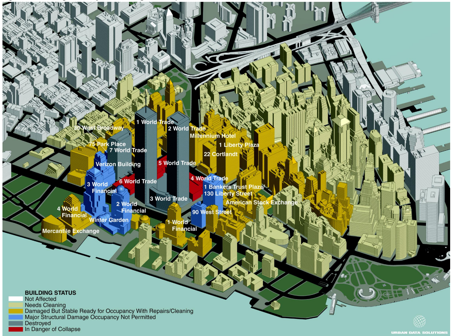
Figure 2: Buildings Destroyed or Damaged on September 11, 2001
