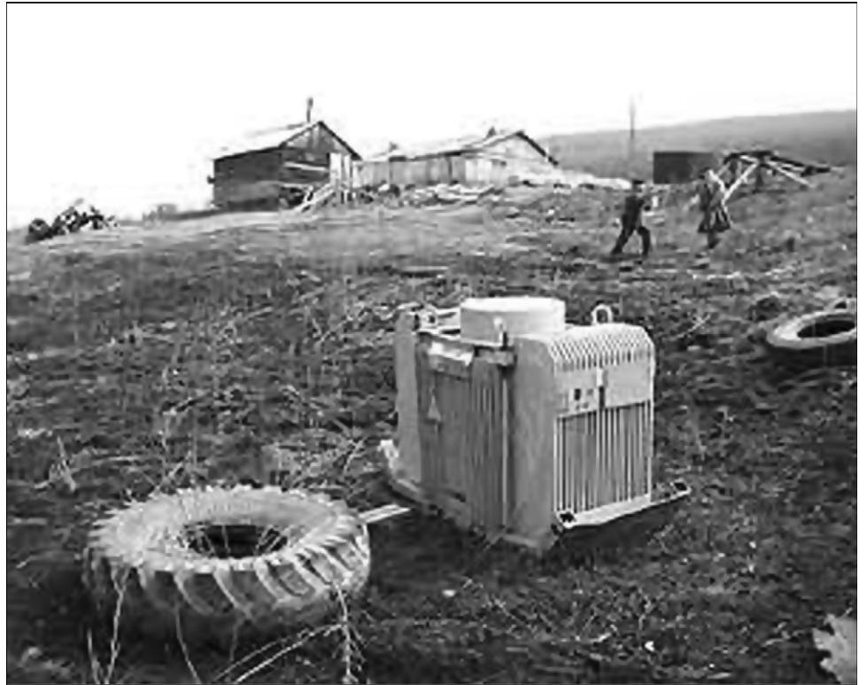
Figure 2: Abandoned Radioisotope Thermoelectric Generator in Russia
