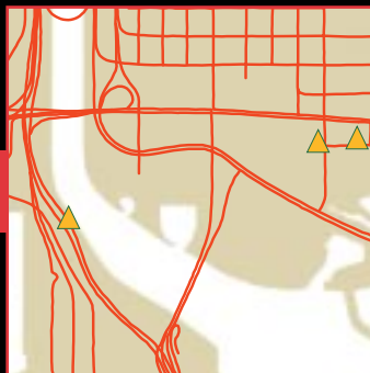
In a stepwise fashion, additional layers are each referenced to NOAA's National Spatial Reference System. Here, the base geodetic control layer, plus the land and water demarcations, are used as a "backdrop" for additional features, such as roadways.
