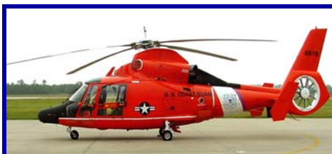
The re-engined HH-65 helicopter successfully completed initial flight testing in Elizabeth City, NC. ARSC/L. Couch
