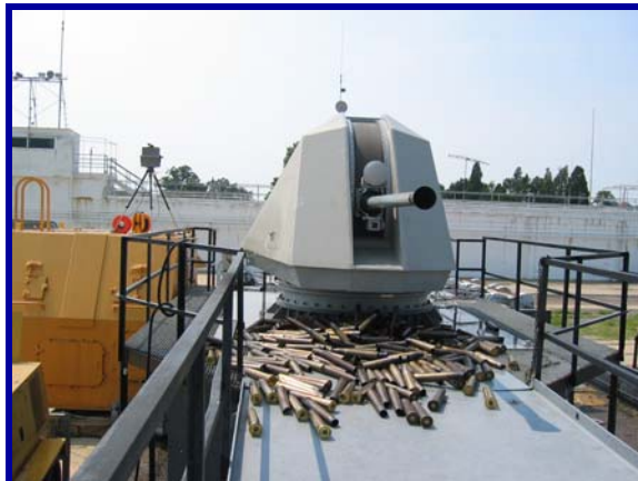
A recent photo of the 57mm Gun Test Fire. Shown is the gun with 120 expended rounds. Photo Courtesy of NSWC Dahlgren
