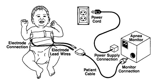
This picture shows the correct way to connect the infant to the Monitor. The ELECTRODE LEADS are plugged into the PATIENT CABLE which in turn connects to the MONITOR. The MONITOR is connected to the WALL SOCKET by the POWER CORD.
