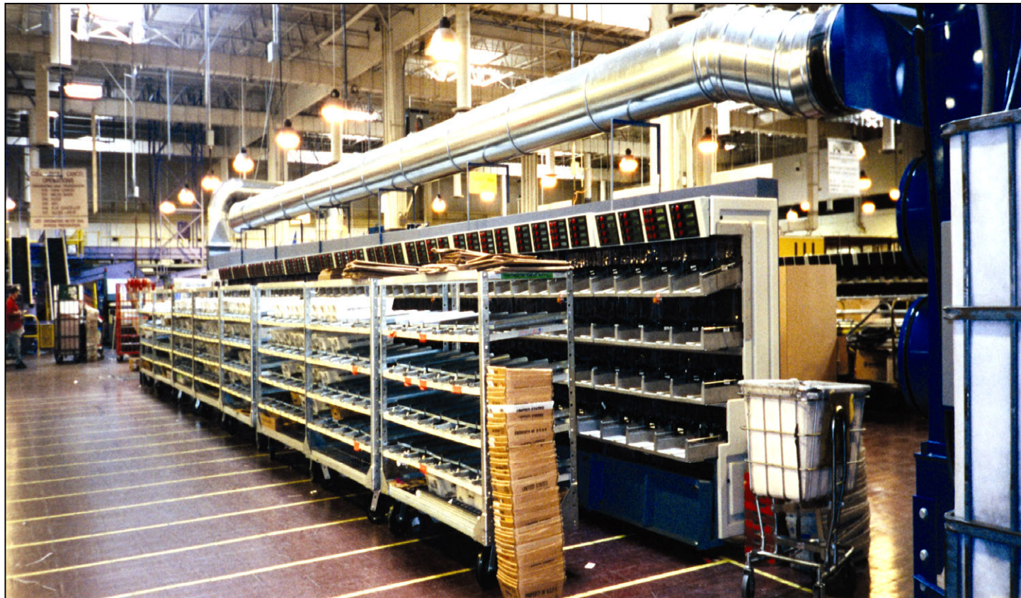
Figure 4: Prototype Torit Air Filtration System on the DBCS
