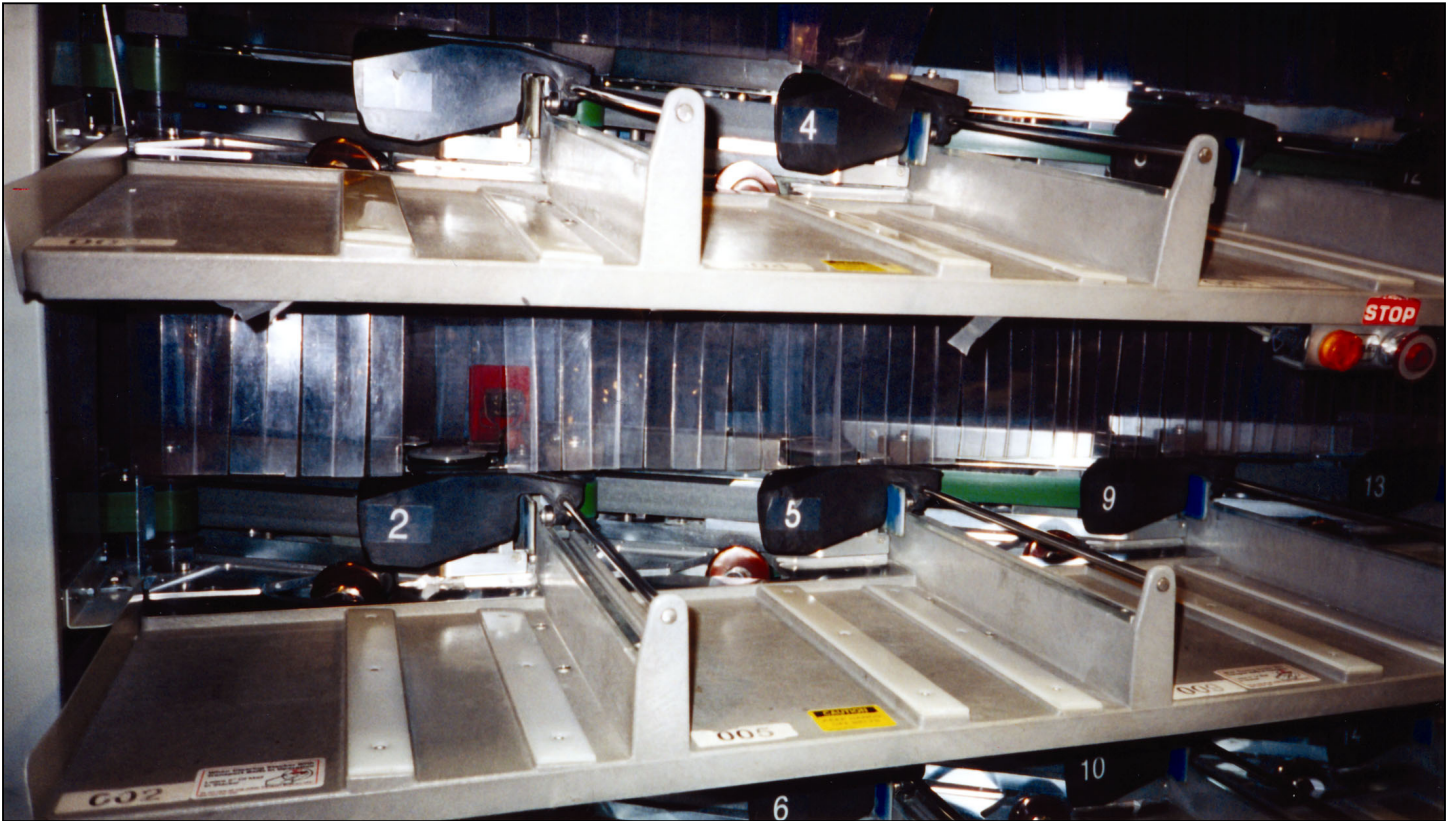
Figure 6: DBCS Modified with Plastic Shrouds
