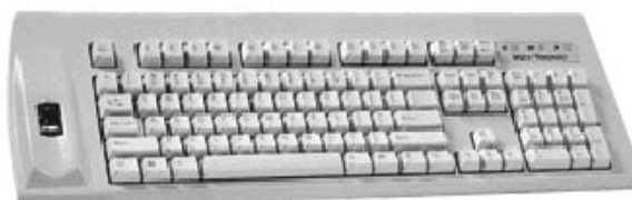
Figure 12: An Example of Fingerprint Recognition Technology Built into a Keyboard
