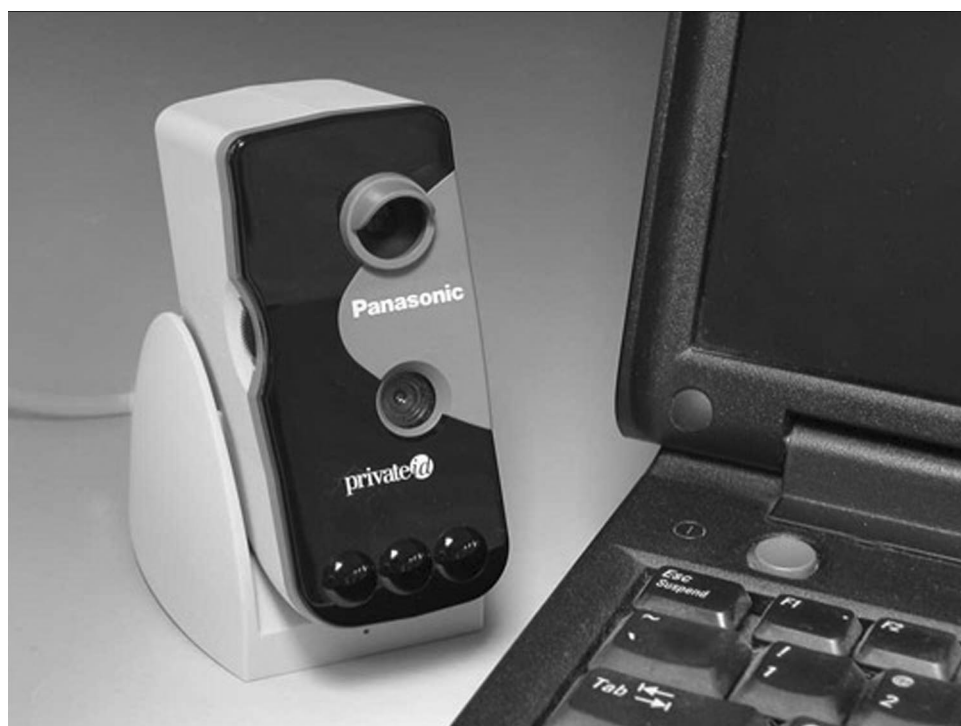
Figure 14: A Desktop Iris Recognition System
