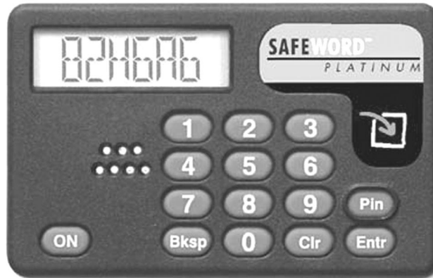
Figure 16: Example of a Challenge-Response Token
