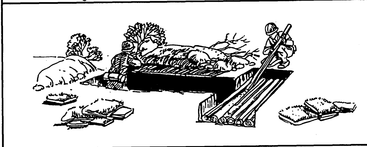
Figure B-28. OVERHEAD COVER SUPPORT LOGS.
