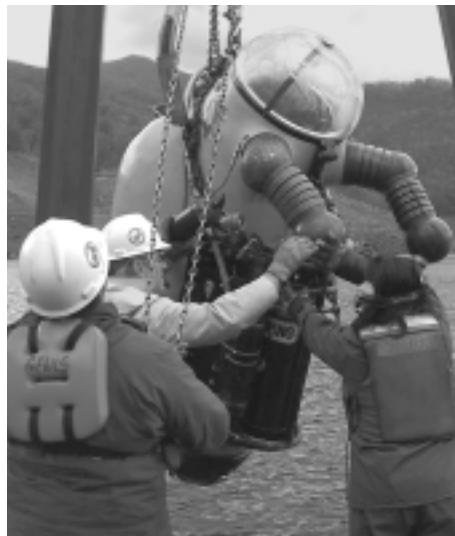
A special “moon suit” was used during the most recent inspection of the outlet tunnel near the bottom of Fontana Dam. The suit enables a diver to work for an extended period at a depth of 200 feet or more.
