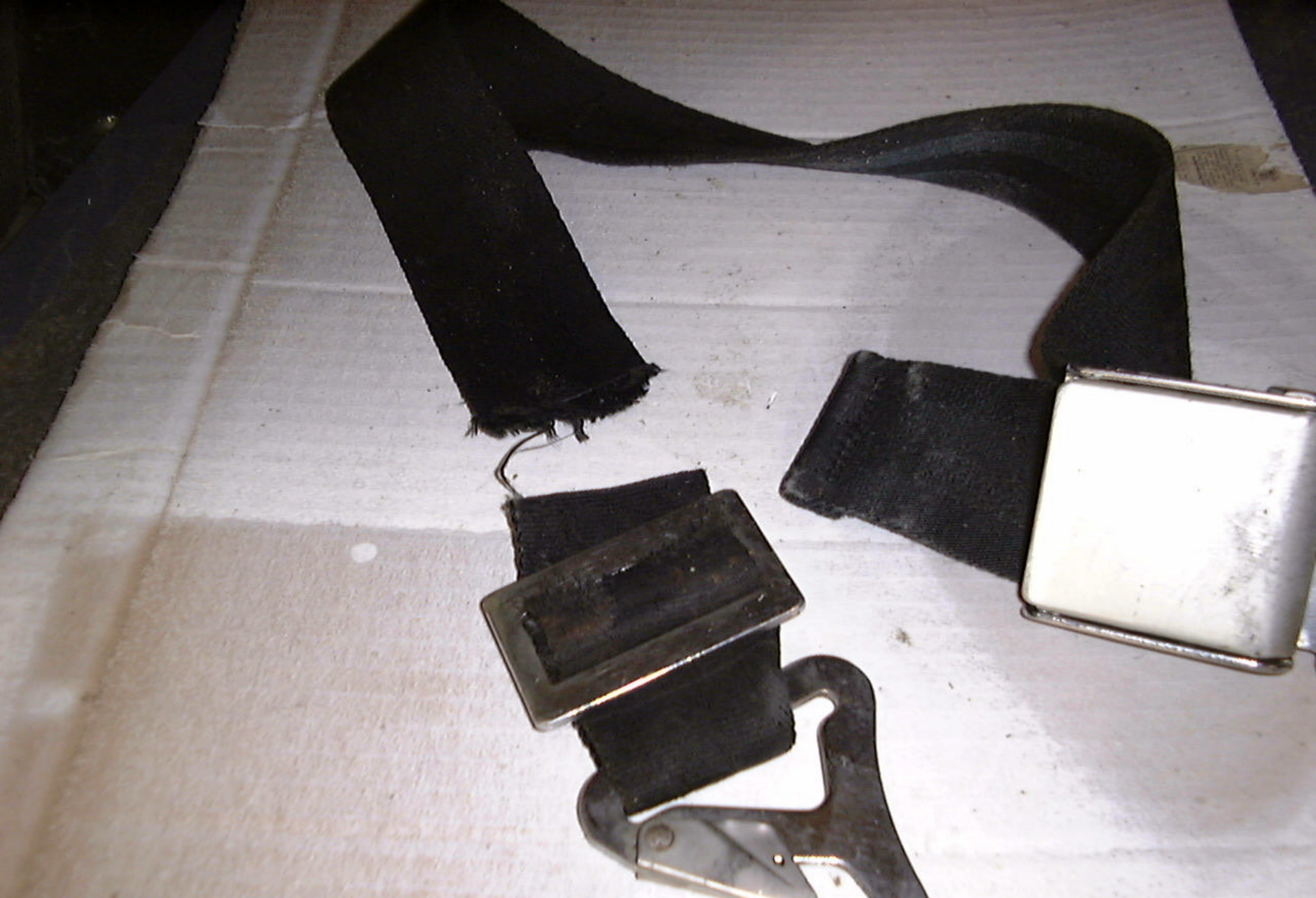
Seatbelt failed during crash sequence
