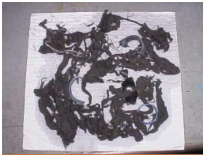
A plane captain found these remains of a rag wrapped around the NR 1 section of the tail-rotor driveshaft.
