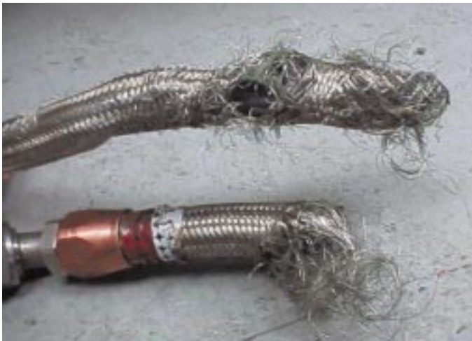
A rag become entangled in the engines' cross-feed fuel lines and damaged them.
