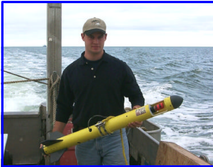
Figure 3-50. Towing package with conductivity, temperature and turbidity sensors.
