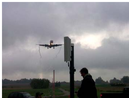
Landing aircraft at St. Louis Int'l Airport create flap vortices near the Volpe instrumentation suite.
