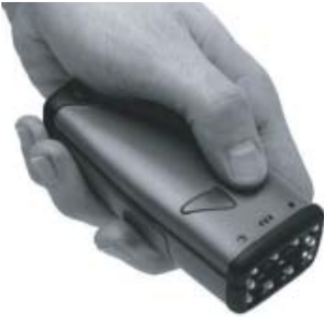
Figure 3: Code Corporation's Code Reader 2.0
