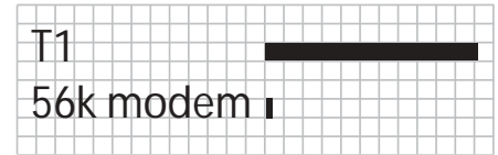
Figure 2: T1 Network Connections are Capable of Rates of 1.544Mbps Versus a Dial-Up Modem That Is Limited to 56Kbps
