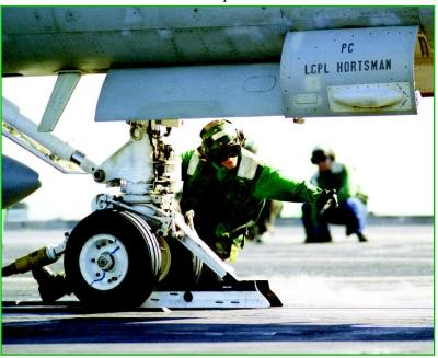
catapult control, relaying aircraft type, gross weight, side number, and catpacity selection valve settings for the launching officer.
