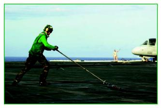
Hook Runners—Ensure cross-deck pendant and purchase cable have been disengaged from the aircraft tail hook, and, when the landing area is clear, they give retract signal to the deckedge operator.
