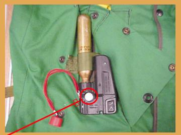
Note the pill used in the new auto-inflator. Order chemical pills in packages of 10: 1701SP1-00-NAV, chemical-pill inflators and gaskets: 1701KIT-00-NAV.
