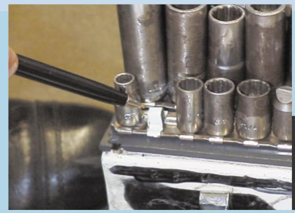
The white paint means the corresponding tool has been surveyed. The document number must be entered on the toolbox's shortage list and filed with QA.
