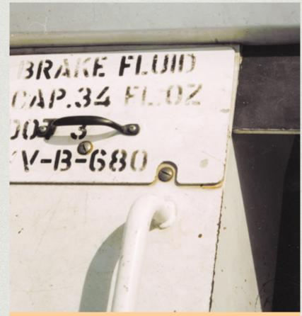
The brake master-cylinder reservoir is the second item most operators can't locate. It's to the right and forward of the driver's seat, under the brake fluid sign.
