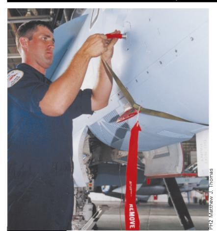
Covers, such as the ones being installed by this Hornet plane captain, keep bugs and dirt out of pitot tubes when the aircraft isn't flying. Pitot tubes get very hot when energized.
