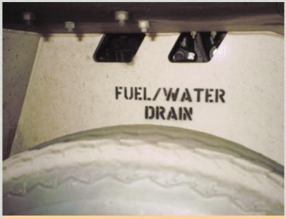
Even though location of the fuel-water separator is painted on the tractor and identified on the pre-op card, most operators don't know where the item is. (It's located on the engine side of the right-front wheelwell.) off the LPO. Not an easy task, but if I'm successful, a mechanically inclined operator eventually will trace the brake lines. If he's really smart, he gives up altogether.
