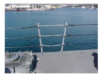
The bracket on the deck and the bracket on the stanchion are designed to have a brace fitted between them to support the stanchion. I have counted as many as 15 missing braces on one ship. Most of the end-run stanchions are bent and the lifelines are slack. If the brace is not in place, then tightening the turnbuckle eventually will bend the stanchion.
