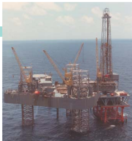
Above: The jack-up rig Rowan Paris drilling for deep gas at depths greater than 15,000 ft below the seafloor. Photo courtesy of The Rowan Companies, Inc.
