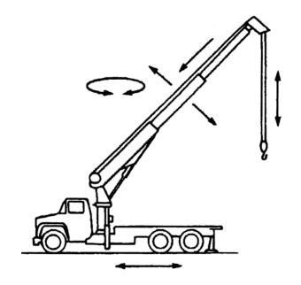
COMMERCIAL TRUCK-MOUNTED CRANE - TELESCOPING BOOM
