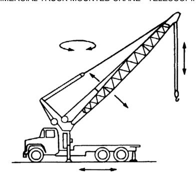
COMMERCIAL TRUCK-MOUNTED CRANE - NONTELESCOPING BOOM
