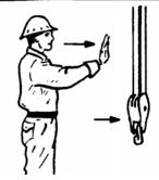
BRIDGE TRAVEL. Arm extended forward, hand open and slightly raised, make pushing motion in direction of travel.
