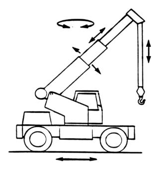
CRUISER CRANE - TELESCOPING BOOM
