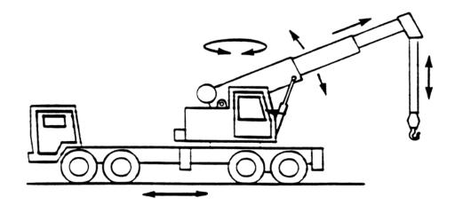
TRUCK CRANE - TELESCOPING BOOM
