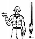
TROLLEY TRAVEL. Palm up, fingers closed, thumb pointing in direction of motion, jerk horizontally.
