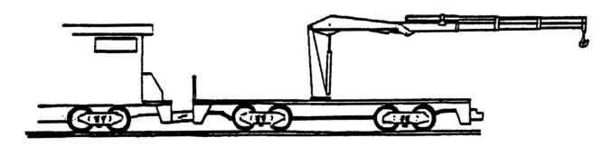
ARTICULATING BOOM CRANE - RAIL CAR INSTALLATION
