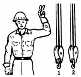
MULTIPLE TROLLEYS. Hold up one finger for block marked "1" and two fingers for block marked "2." Regular signals follow.
