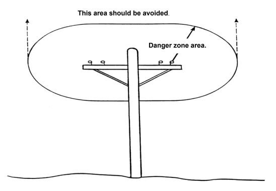
Required clearance for normal voltage in operation near high voltage power lines and operation in transit with no load and boom or mast lowered.
