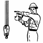
MOVE SLOWLY. Use one hand to give any motion signal and place other hand motionless in front of hand giving the motion signal. (Hoist slowly shown as example.)
