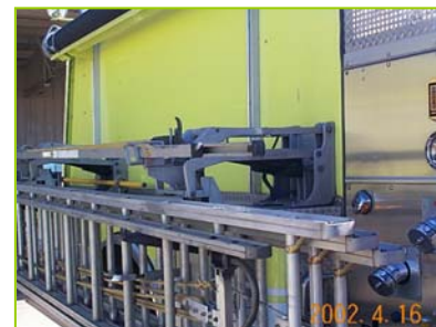
After: Mechanical ladder loader
