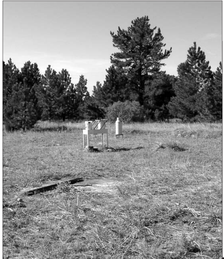
A National Atmospheric Deposition Program wet deposition sampler. Wet deposition refers to acid fog, rain, and snow. This unit was set up in Newcastle, Wyoming, to follow air quality impacts in the area.
