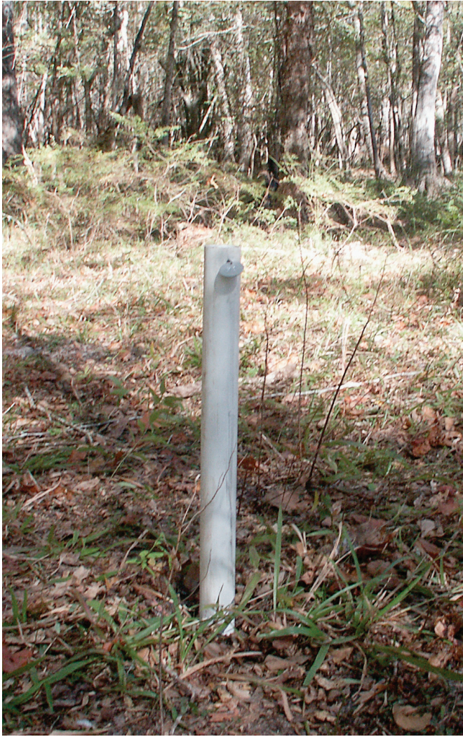
Figure 3. Permanent marker with PVC sleeve used to mark transects in the lower Suwannee River floodplain, Florida.
