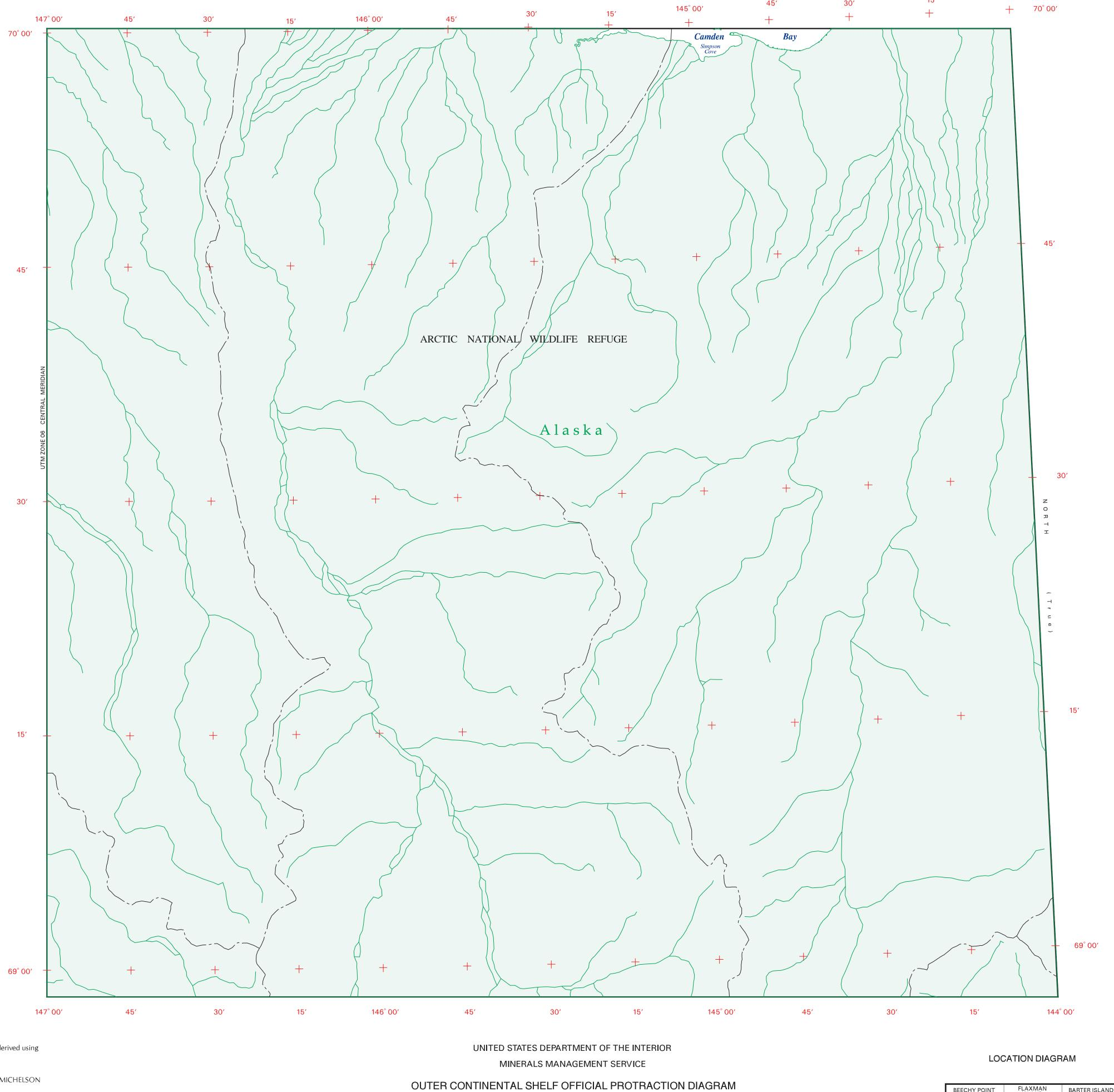
The boundaries of the regular blocks are 4,800 international meters on a side and contain 2,304 hectares. The regular boundaries are defined in terms of X and Y coordinates of the Universal Transverse Mercator Grid System based on the Geodetic Reference System (GRS) 1980 Ellipsoid.
