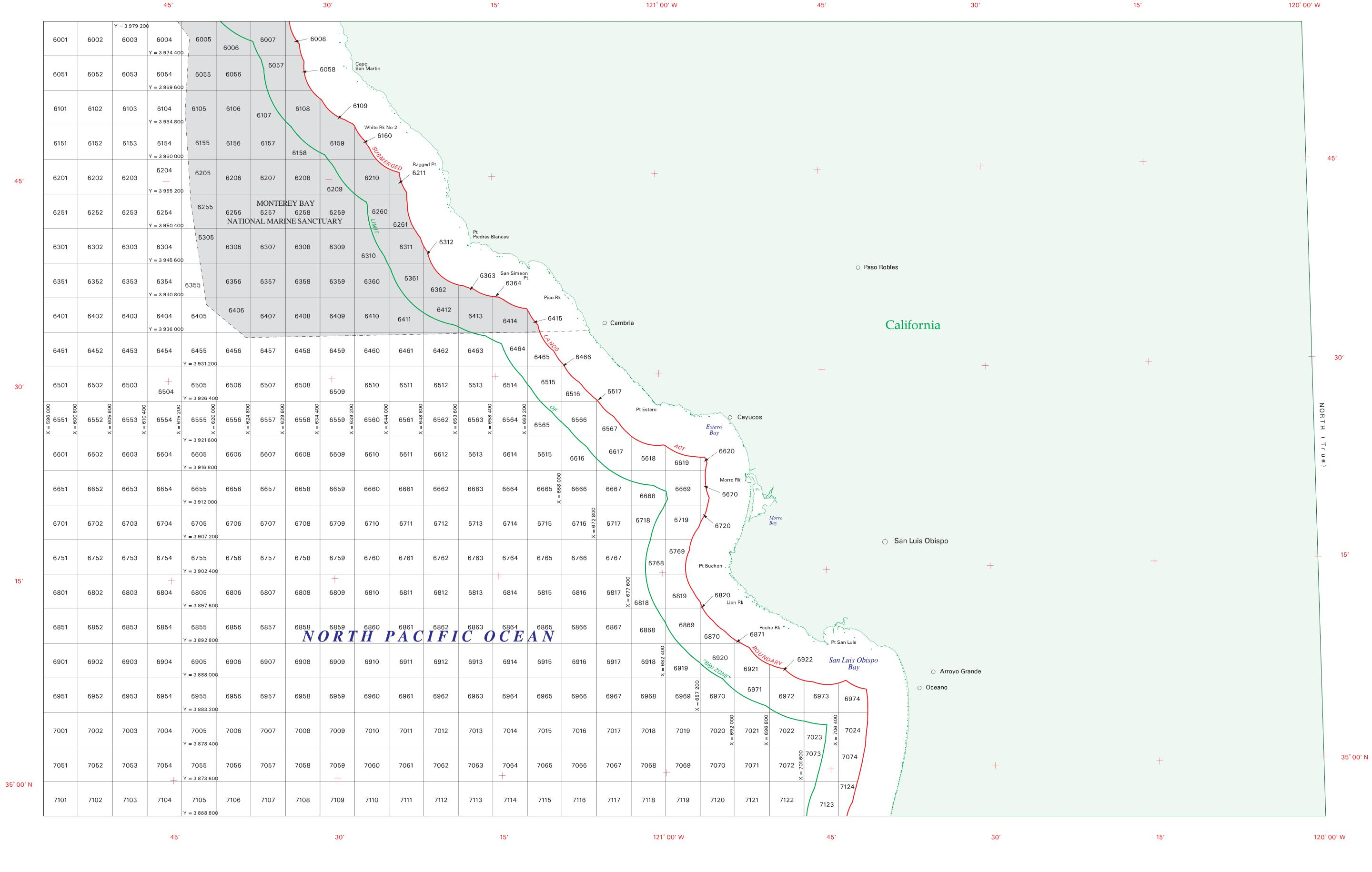
The boundaries of the regular blocks are 4,800 international meters on a side and contain 2,304 hectares. The regular boundaries are defined in terms of X and Y coordinates of the Universal Transverse Mercator Grid System based on the Geodetic Reference System (GRS) 1980 Ellipsoid.
