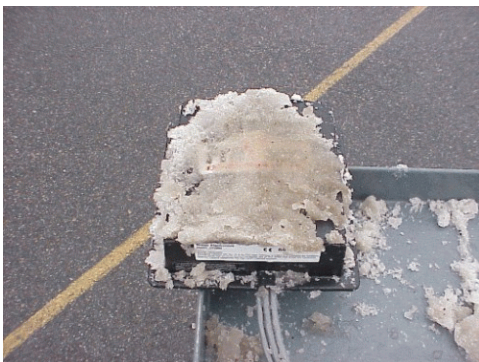
Figure 13.—Thin layer of snow on Preview radar, which caused an alarm.
