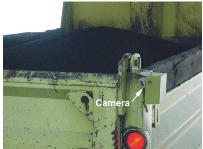
Figure 21.—Final installation of Intec camera on dump truck.
