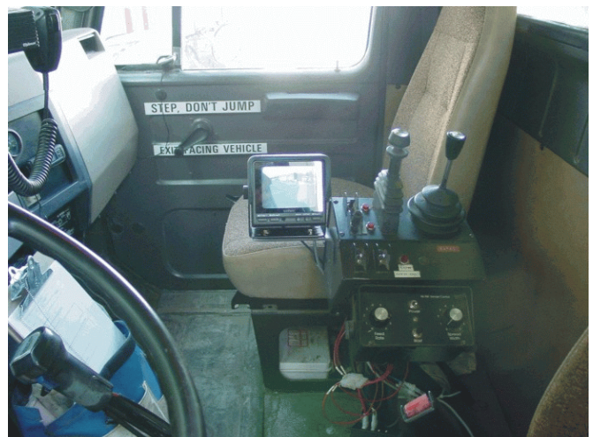
Figure 22.—Intec monitor installed in truck cab.
