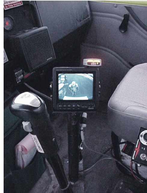
Figure 10.—Clarion video monitor with Preview alarm display mounted on top.
