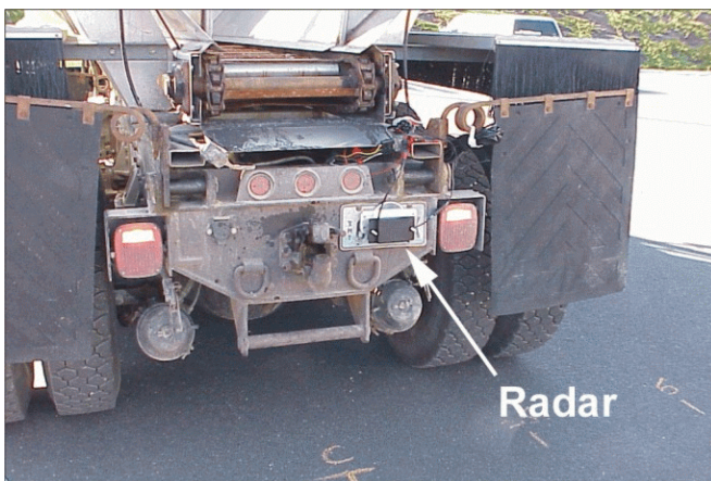
Figure 4.—Guardian Alert radar system on sanding truck for short-term test.
