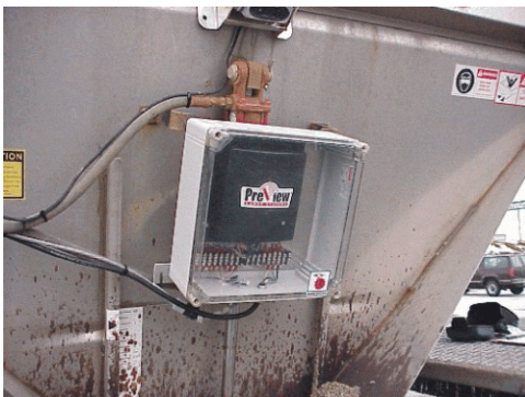
Figure 9.—Final mounting of Preview radar system on sanding truck.
