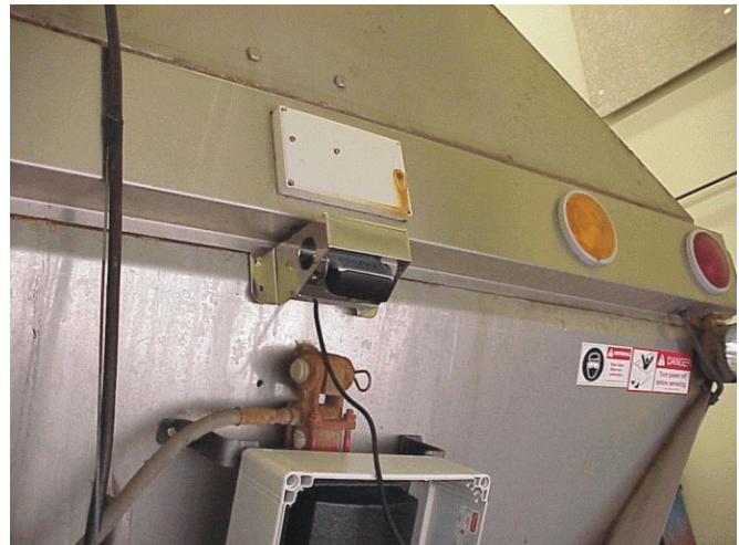
Figure 17.—Clarion camera mounted on back of sand hopper.
