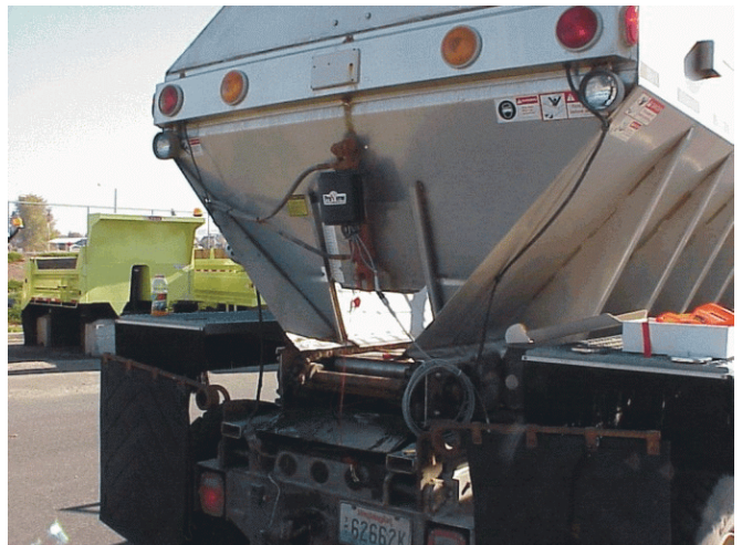
Figure 7.—Preview radar system mounted on sand hopper. height, a crouching person might not be detected immediately next to the tires, and the tilt of the radar would need to be increased if possible.
