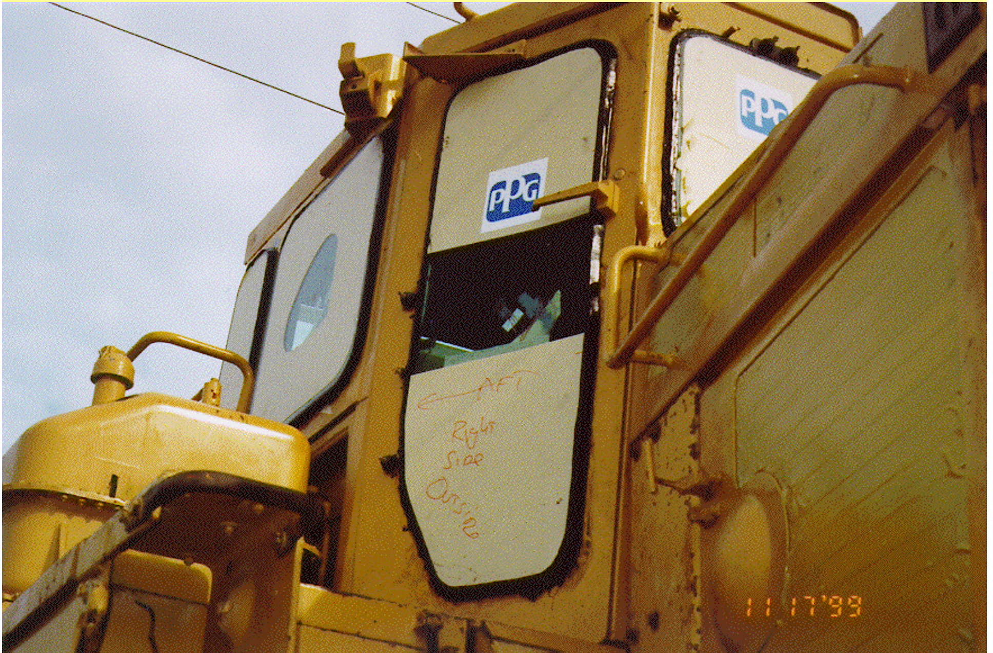
High-strength glass installed in all cab windows of test dozer.
