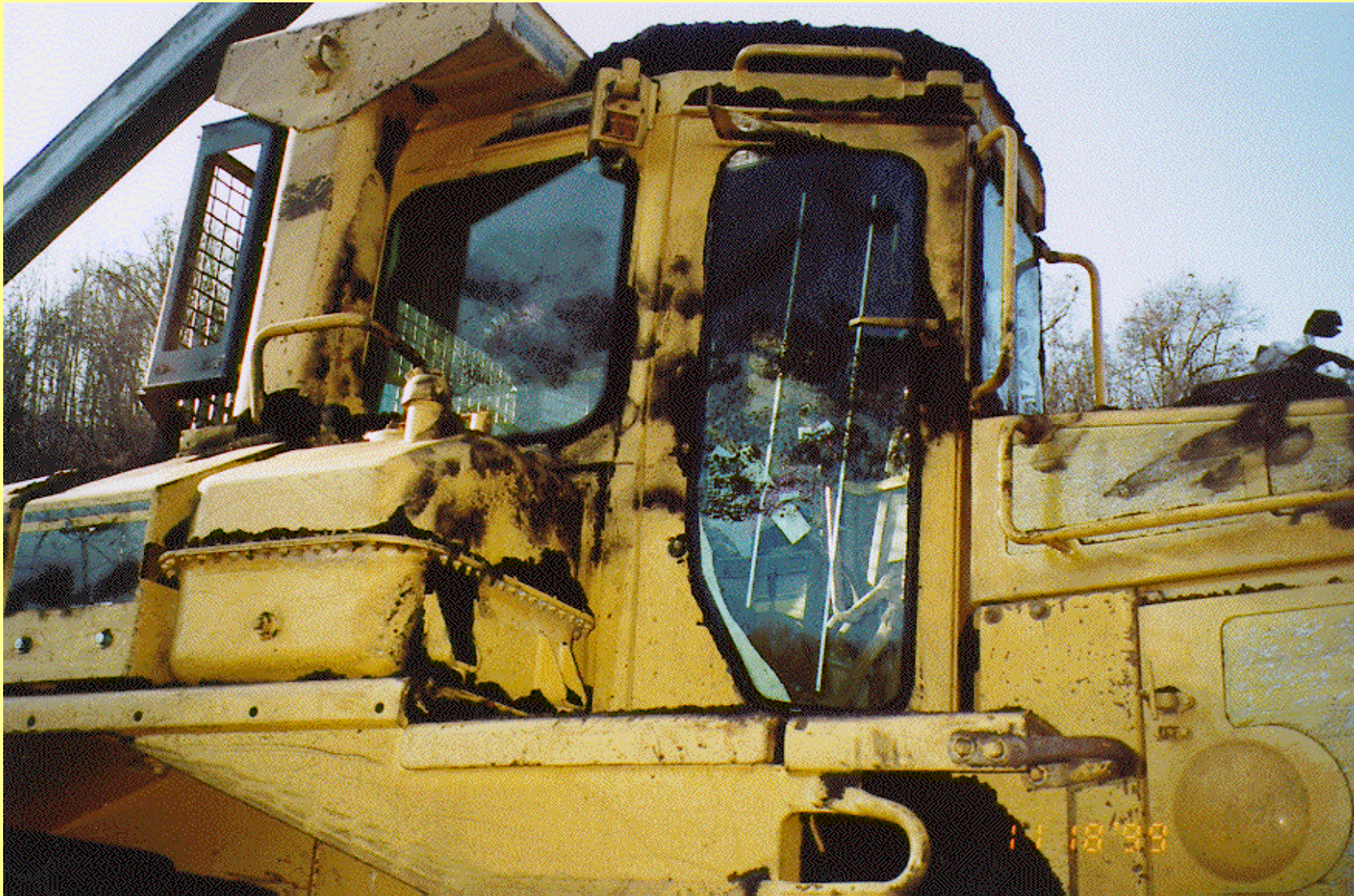
High-strength glass intact after burial demonstration.
