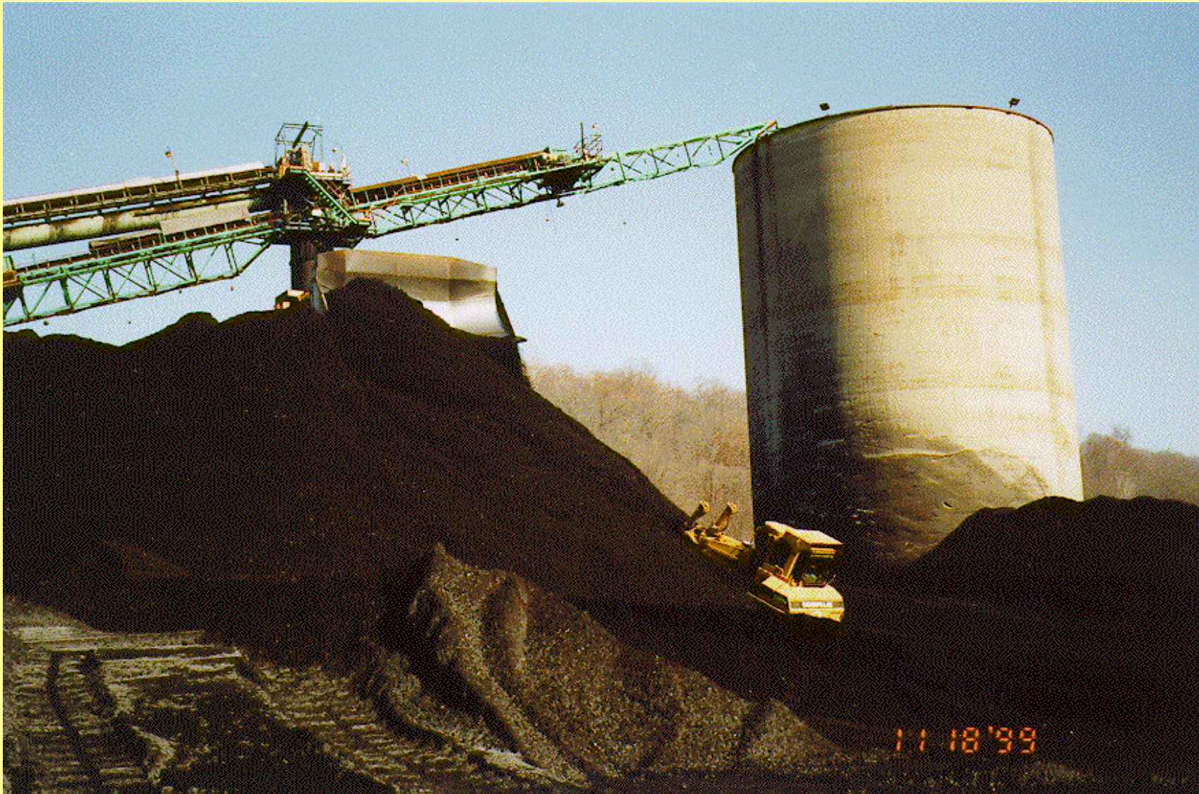
Dozer with high-strength glass being buried in coal pile...
