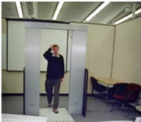
The system provides a graphical interface to the operator by using freeze-frame video capture technology, and places filled circles – dependent upon the number of items detected – over the video image indicating where suspected weapons may reside on a person (photos at left). The detector uses 16 magnetic gradiometer sensors, arrayed on both sides of the portal aperture (detail below).
