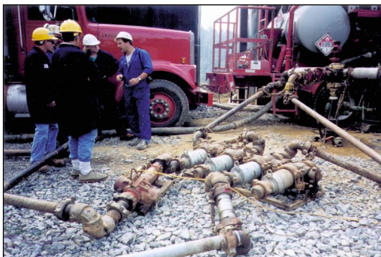
Figure ES-6. The fracturing fluids, additives, and proppant are pumped from the storage tanks to a manifold system placed on the wellhead where they are mixed just prior to injection.
